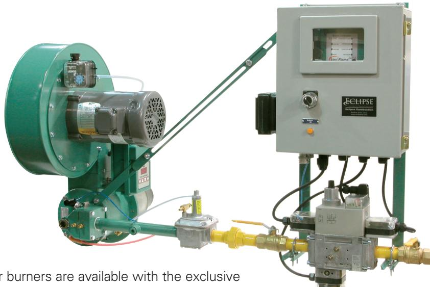
All RatioAir burners are available with the exclusive HeatPak packaging option. Each packaged burner unit includes an Eclipse Veri-Flame modulating single burner monitoring system, valve train, gas pressure switches, position indicator and ignition transformer with a metal NEMA 12 enclosure. All piping and wiring to supply a completely operational unit that meets NFPA-86 standards is done at the Eclipse factory. The customer connects gas and electricity and the burner is ready for operation.
